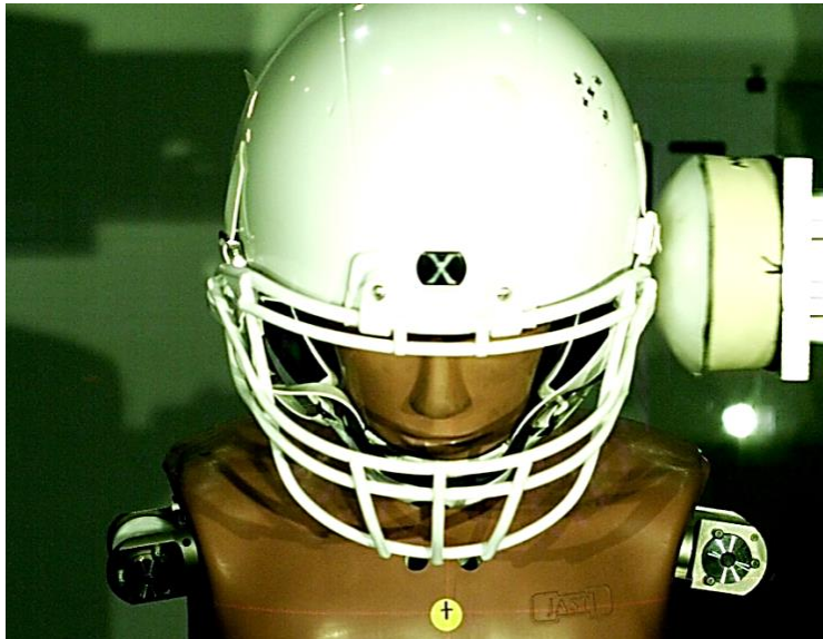
Figure 5.3 – Sample test setup to assess the repeatability of the impactor system when used in a ram configuration striking a stationary helmeted ATD.
