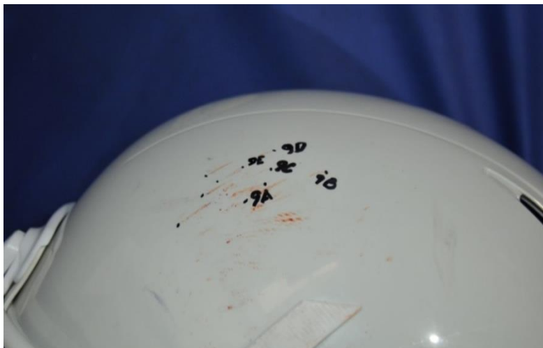
Figure 5.6 – Impact location on helmet of ATD on impactor 2 from a set of five tests with two moving ATDs.
